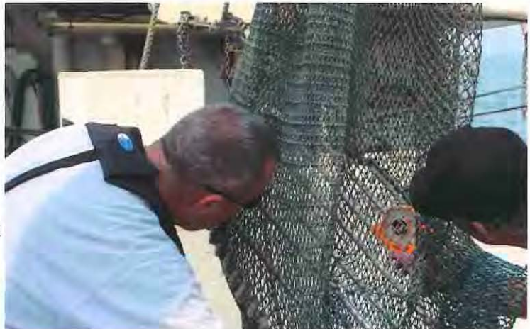
A NOAA special agent and a state partner check the angle of a Turtle Excluder Device. TEDs education and enforcement are a high priority for NOAA's Office of Law Enforcement's Southeast Division.
